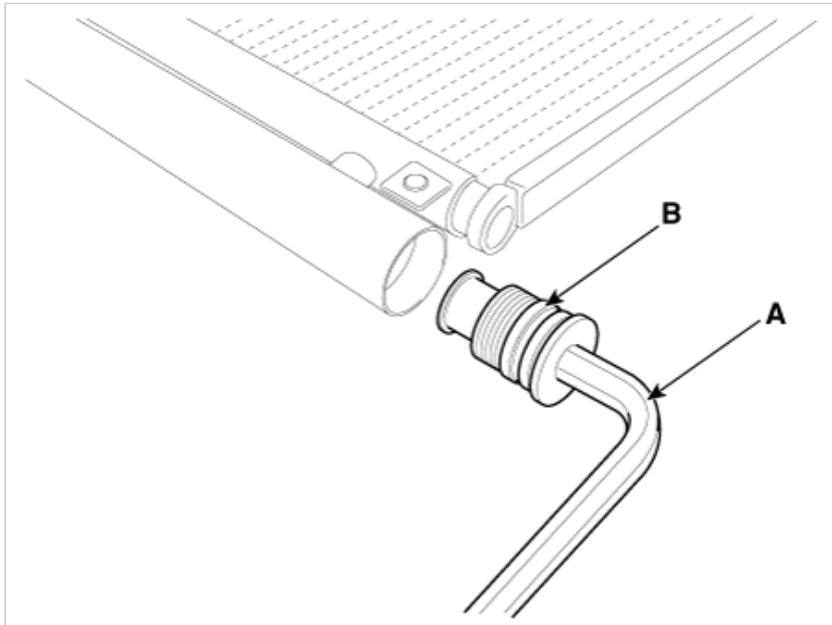
3. Remove the receiver-drier (A) from condenser using long nose pliers. Check for crumbled receiver-drier and clogged bottom cap filter.
