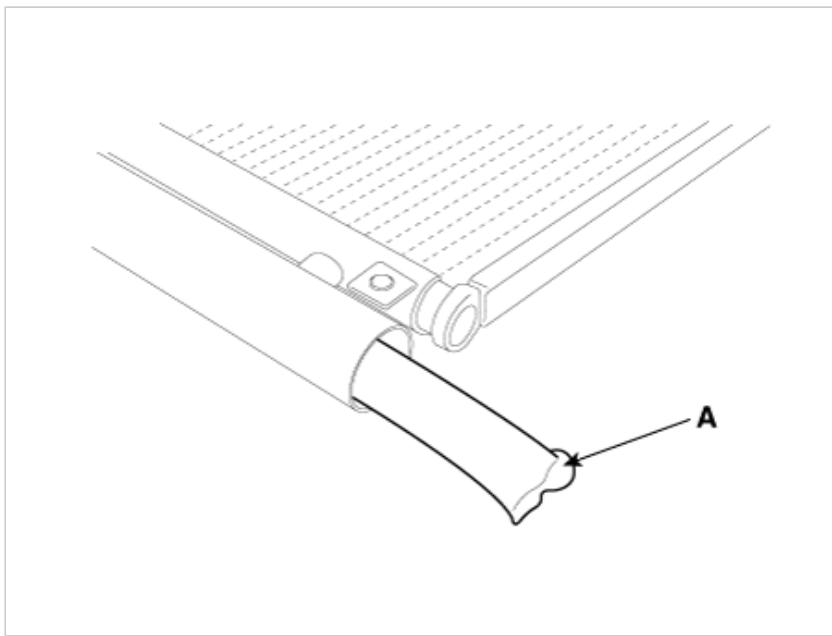
4. Apply air conditioning compressor oil along the O-rings and threads of the new bottom cap.
